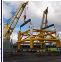
panish freight forwarder Altius Projects Division performed a part-cargo of a jacket plus additional equipment on board the vessel Trina for a trip between Aviles and Grenada. The size of the jacket was 30m long by 27m wide by 15m high with a weight of 576 tons. www.gpln.net
