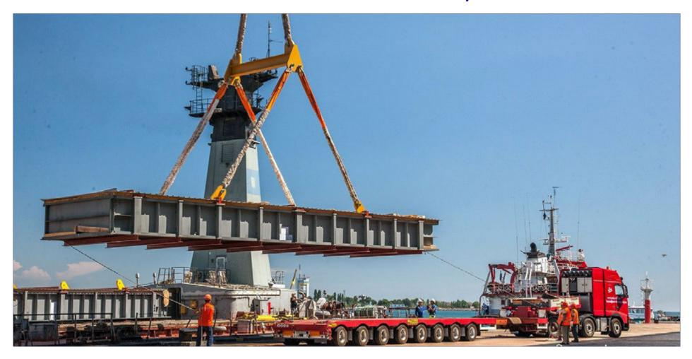
or a fertilizer plant being built in the southern part of the Ukraine, DAKO Worldwide Transport GmbH Düsseldorf recently transported seven modules with unit weights between 100 and 130 tons, each from the factory in Italy via the port of Chioggia to Yuzhny near to Odessa
