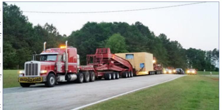
rated several bridges, so extensive bridge engineering studies and route surveys had to be done prior to the move. Both the bed and crown required night moves and the 500-kilometer trips were completed in just two nights.
