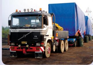
The main compressor unit was 48.00 metric ton each and had dimensions of 12.45 m x 3.25 x 4.01 m.
