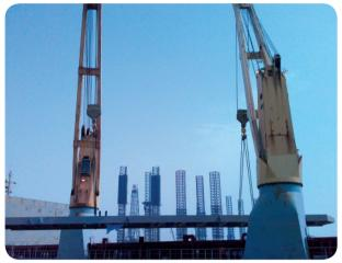
alongside the vessel with dims of 38.43m long, 5.8m high, 1.8m width and weight 160 mt.
