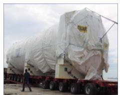
Due to the nature and size of the cargo there were different modes of transportation used. The journey started from Italy via chartered vessel to Malaysian West Port, then discharged to a multi-axle trailer for another journey to a private jetty were the cargo was rolled onto a 250-feet barge sailing to Melacca.
