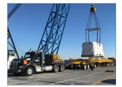
shipped to the port of Savannah that had to be delivered in conjunction with the breakbulk pieces. The final 113,000-kilogram lower-bed transport required months of planning and was moved using a specially designed beam dolly trailer. They had to move at night from Virginia to the North Carolina border.
