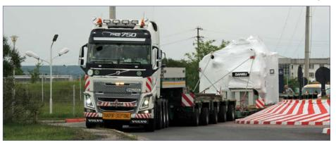
low beds with 12 axles 35 centimeters from the ground for the transport. The two pieces together with two hydraulic cylinders, each weighing 33 tonnes, were unloaded and assembled in Slatina by the heavy lift division of Holleman in a nine meter high hall. In order to
