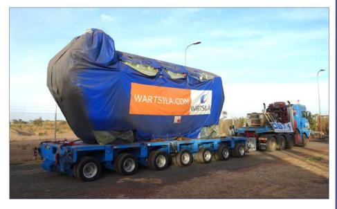
DAKO was responsible for the reception of the engine in the port of Banjul, reloading from MAFI trailer onto hydraulic trailer, the overland transport up to the jobsite and for the exchange operation inside of the power house.
