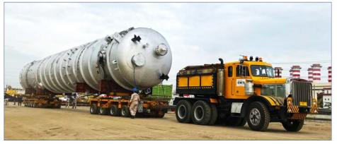
To achieve this seamlessly, CKB Logistics provided project logistics services to deliver the naphtha splitter column to Pertamina RU IV- Cilacap site. The mobilization was arranged with a combination of prime mover 6x4, multi-axle with 10-axle line and baby bed to transport the column.
