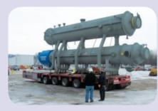
Typically these units are shipped separately due to the excessive height restrictions. These shipments were the largest design component ever shipped piggyback style by Selas Fluid Processing which resulted in a major cost savings for transport and field installation related expenditures.
