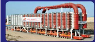
Huge evaporators are very important for the project. three sets of signal lights for each move. length, 22 meters width & 13 meters height.
