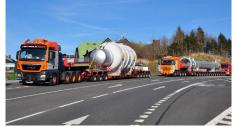
roads with this heavy load on board. The plant components impressed with their dimensions, heat exchanger number 1 weighed a whopping 118.4 tons with a length of 22.43 meters, a width of 2.88 meters and a height of 3.21 meters. Heat exchanger 2 – at 59.85 tons almost a light weight – was "only" 10.39 meters long, but 3.89 meters wide and 4.5 meters high.
