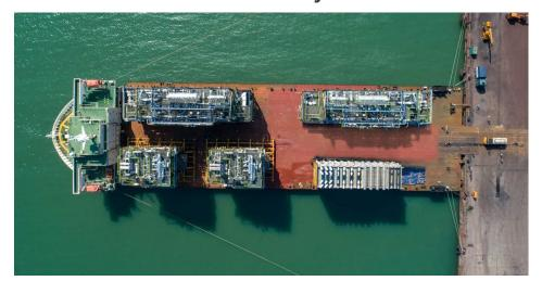
PLN member Lift & Shift (LSPL) delivered the biggest, heaviest boiler & HRSG modules built in India by Thermax for the largest refinery in Nigeria. Thermax was awarded one of its largest export orders for a large refinery project coming up in Nigeria. Thermax assembled all the plug & play modules in its modularization yard at Mundra SEZ & delivered all the modules from Mar'19 to Nov'19. Thermax delivered 8 x HRSGs, 4 x UBs and 2 x FGSG modules.
