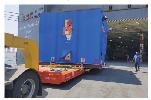
metres alone, the height of the unit was too high for transhipment operations. Most of the vessels in the Middle East to India and Africa service have a door opening of around 5.0 metres so the solution was to use Hbegh's Superlow rolltrailer. The Superlow rolltrailer is only 0.47 metres high and is designed to load Breakbulk cargo that is
