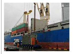
HIREY Projects from China recently shipped a power plant from Shanghai to Chattogram (Chittagong) in Bangladesh. The commodity was transformers with a measurement of (each) Length: 9,10m / Width: 3,26m / Height: 4,10m and Weight: 140 tons. The service including inland transportation, customs clearance, chartering of heavylift vessel and so on.
