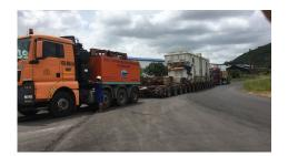
n July 27th, 2020, Vietranstimex successfully received and transported the 220kV-250MVA Transformer (measuring 11,83m x 3,23m x 3,62m) with a weight of 140 tons and associated fuels and fittings of 95 tons from 220kV Than Uyen Substation (Lai Chau) to 220kV Thuy Nguyen Substation (Hai Phong).
