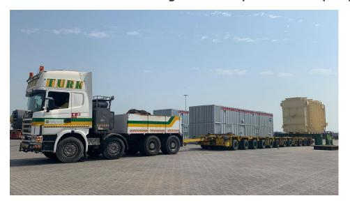
urk Logistics & Heavy Transport from the Kingdom of Bahrain, recently completed another successful barging operation. The shipment consisted of one unit of a transformer, with a weight of 140 tons and dimensions of 8.70m x 3.55m x 4.40m (L x W x H). During the arrival of the shipment in Bahrain, Turk team received the transformer from ship hook and placed it on the stools support to complete the customs formalities.
