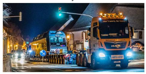
For the road transport of the locomotive, however, many traffic control measures were necessary along the 360 kilometers to Hamburg, traffic signs were dismantled, trees had to be cut, roadway plates were laid out and curve radiuses expanded. The height of the transport – the locomotive plus the low-loader measured an impressive 4.50 meters – posed a major challenge. When crossing bridges, there was often
