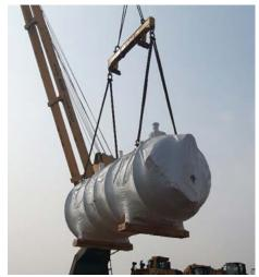
filters, all measuring over 5 meters in height, from FCA Milan in Italy to Stettin in Poland. The cargo was moved by road from Milan area to Porto Marghera and safely loaded on board M/V Nauma to Poland. Lysander had to apply for permits for road transport through 5 different counties in Italy and co-ordinate safe arrival to Porto Marghera, just in time to meet the scheduled part charter vessel.
