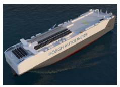
our fleet. This has put us in the forefront in sustainable shipping in the deep-sea RoRo segment. The Aurora class is designed to transport the cargo of the future. Its strengthened decks and enhanced internal ramp systems, enable Electric Vehicles on all decks and provides more flexibility for heavier project cargo.
