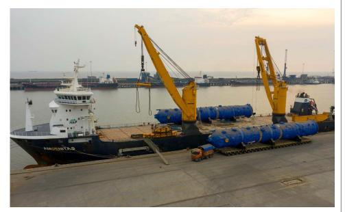
PLN member Total Movements from India stepped up to the plate and recently moved Contractors for a prominent export project in the Middle East. As part of this project, Total Movements successfully delivered two 552MT/44-metre—long MDEA Contactors (Super ODC) from the supplier's works to the load port on the west coast of India. With the critical cargo dimensions in mind, this movement was meticulously planned.
