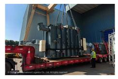
Tanks from Shanghai to Kaohsiung, Taiwan, by chartering a breakbulk vessel. The dimension and weight of the largest one was 16,770\*4,100\*4,000 m and 4,3202 kg. The total volume of the lot was 165 CBM / 176.72 tons.
