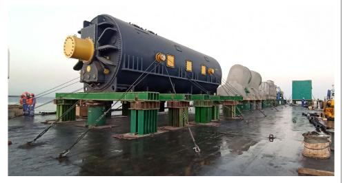
PLN member Turk Logistics from Bahrain performed a multimodal transportation of 14 units of a Steam Turbine Generator and Generator Step-up transformer for a Water and Power Plant in Bahrain. As part of this project, Turk Heavy Transport successfully delivered several of these units with a weight range from 207 MT to 343 MT per piece.
