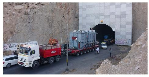
the aforementioned task of delivering 02 heavy-lift transformers main bodies, weighing 120 tons each and dimensions as 9.35 x 3.76 x 4.21 meters, MAMQ first conducted the land route physical inspection survey from Karachi Port (Origin) to Quetta Grid Station (Destination) via RCD road to understand and form-up the strategy and provide solutions for the challenges & hindrances existing enroute.
