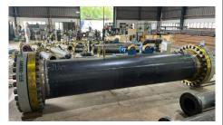
PLN member Megalift sent a large and heavy spool by air freight from Kuala Lumpur / Malaysia to Denmark for repair and maintenance purposes. The spool had a dimension of L4.17 m x W1.44 m x H1.52 m and a weight of 4 tons. Their client uses the spool for calibration purposes, and it required some urgent fixing. The repair work took three weeks, and Megalift arranged also the return shipment from Denmark to Malaysia by air.
