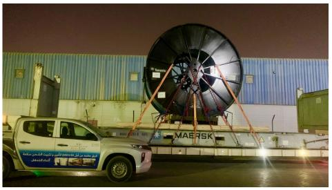
possible by loading a 41-ton Coiled Tubing into a heavy-duty 40' Flat Rack container, pre-lashed and safely loaded from Jebel Ali to Europe.
