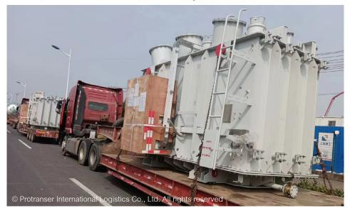
PLN member Protranser's team from China delivered recently 2 sets of 54.8 tons transformers from Shanghai, China, to South Asia. The dimension of the main body was 5,00\*3,15\*3,35 m. Working scope was chartering service of breakbulk vessel.
