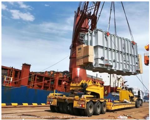
PLN member Protranser from China delivered recently 2 sets of 127-ton transformers from Qingdao, China, to Canada. The total volume was 36 pieces / 326 MT / 613 CBM. Working scope was local picking services, port service in Qingdao port and booking procedure.
