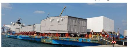
ur GPLN member from UAE, Fleet Line Shipping, has recently made a move-ment involving 4 x modules measuring up to 37 m length x 15.54 m width x 8 m height and weighing up to 450 MT each. The modules were brought from the fabricator yard in Hamriyah FZE to Hamriyah, Sharjah port, using 104 axle-SPMT's. Several temporary civil work modifications had to be done, including temporary removal of electric posts & sign boards. The modules were eventually loaded using the RORO method on a deck carrier.
