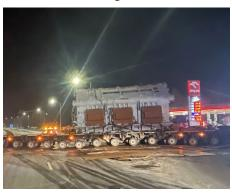
n February 2025, GPLN member Baltkonta UAB from Lithuania successfully launched a large-scale transportation project. A 200-ton transformer was being transported over a 645 km route on Lithuanian roads, with the estimated delivery to the final destination by the end of March – beginning of April.
